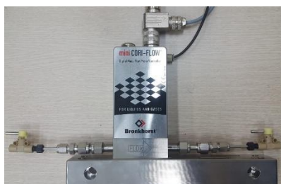
Figure 2: Coriolis flow meter including mass block from Bronkhorst High-Tech.
