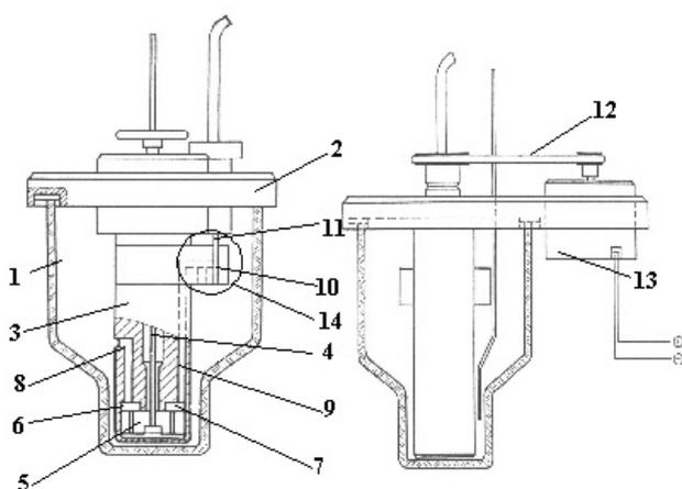
Fig. 2. Electrochemical vessel structure
